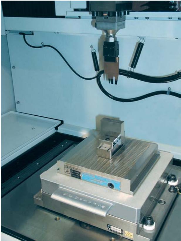
Permanent magnetic chuck for electric discharge machine
