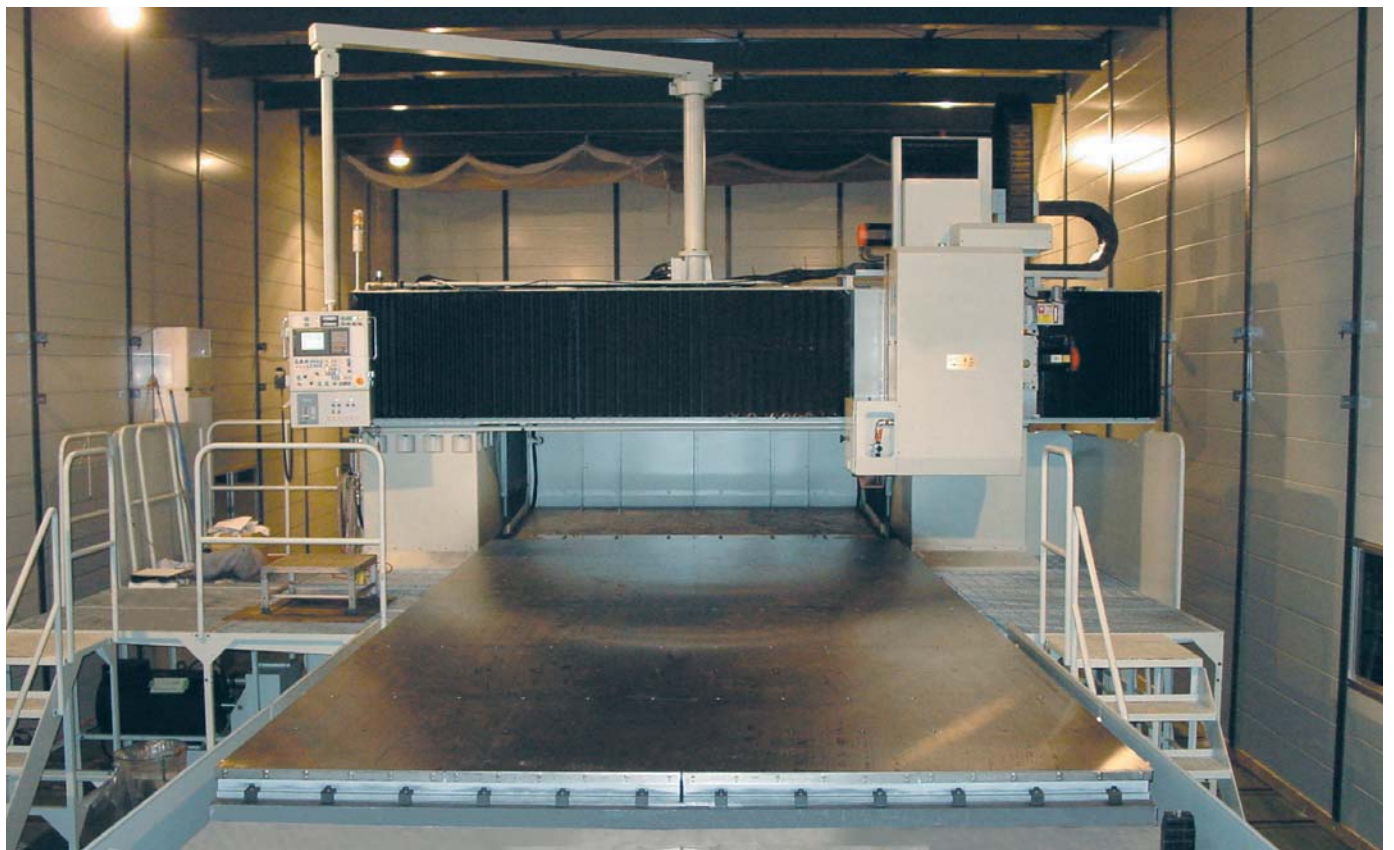
Permanent electromagnetic chuck for grinding (An example of large-size fabrication)
